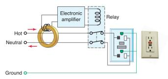
Zero current flows in this conductor under normal operating conditions.
