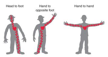
**Figure 1-2** Typical electric current pathways that stop normal pumping of the heart.
