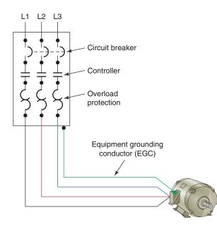
Figure 1-10 Equipment grounding conductor (EGC).
